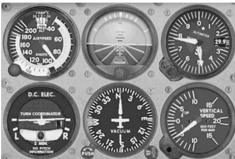
Figure 2-7 Primary Instruments for an ILS Approach. Airspeed, primary for power; Directional Gyro, primary for bank; Vertical Speed, primary for pitch.
